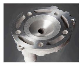
The head above had detonation damage that was repaired by welding and machining.
